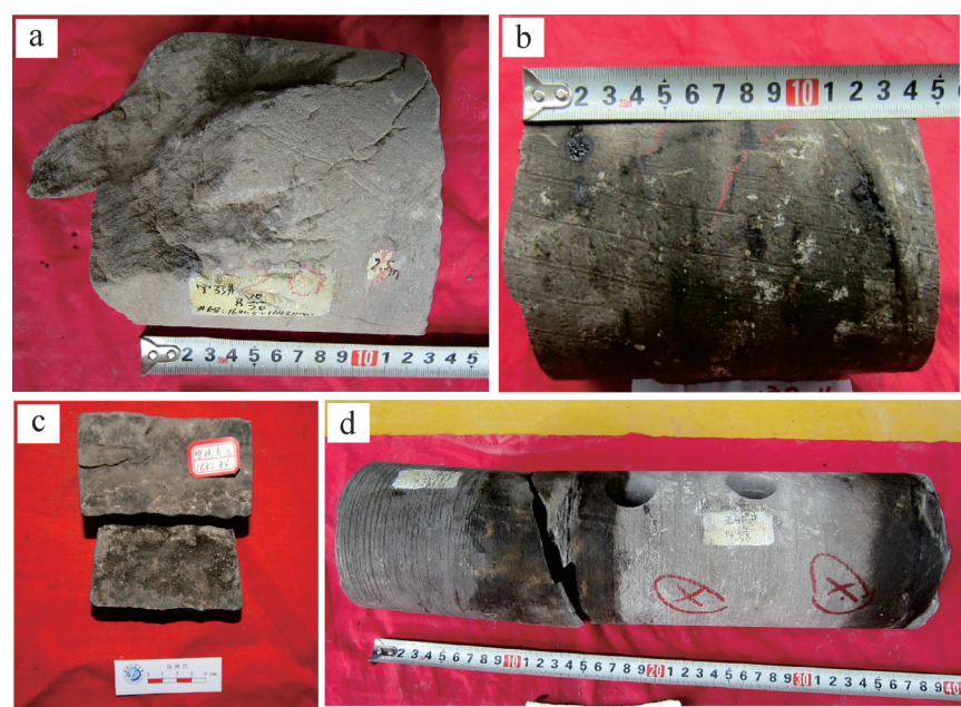
图 14 正宁地区长7段含裂缝岩心照片 (a)N33井,长7 1 亚段,致密砂岩储层高角度构造缝;(b)N80井,长7 2 亚段,致密砂岩裂缝充填原油;(c)N33井,长7 2 亚段,粉砂质泥岩高角度裂缝面,被原油沾染,含油性明显;(d)Z40井,长7 2 亚段,致密砂岩裂缝含油 Fig.14 Fractured core photos of the Chang 7 member in the Zhengning area (a) well N33, Chang 7 1 sub-member, high angle structural fracture of tight sandstone reservoir; (b) well N80, Chang 7 2 sub-member, tight sandstone fracture-filled crude oil; (c) well N33, Chang 7 2 sub-member, silty mudstone high angle fracture surface, contaminated by crude oil, oiliness is obvious; (d) well Z40, Chang 7 2 sub-member, tight sandstone fracture oil
